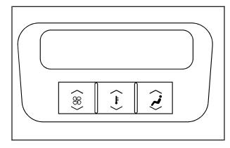
If your vehicle has a rear climate control system, the rear seat passengers can adjust the direction of the airflow, fan speed and temperature for the rear seating area. This system also works with the main climate control system in the vehicle. The control panel for this system is located on the back of the center console.
